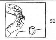
If the eyepiece is too small to fit snugly in the brass tube, wrap it in a layer of two of corrugated cardboard.
