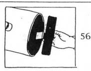
Adjust the spider so that the diagonal mirror is in front of the eyepiece hole. (The diagonal mirror should be facing the hole.)
