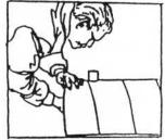
When we look through the eyeplece hole we we should be able to see the reflection of the (open) bottom end of the telescope tube in the diagonal mirror.
