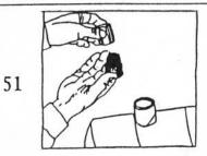
Fitting the eyepiece inside the brass tube. You can purchase an eyepiece, or salvage the eyepieces out of an old pair of binoculars. (See page 4.)
