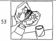
Adjust the amount of cardboard as needed so that the fit of the eyepiece in the brass tube is snug.
