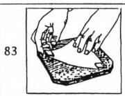
This cardboard protects the mirror from the taligate boits if the telescope is dropped on its end. This cardboard <u>must be floopy</u> so as not to reposition the objective.
