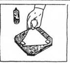
...and glue squares of Masonite (about 1" square) onto the cardboard directly over the protruding bolts.
