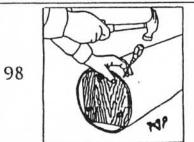
Making pilot holes for the four tailgate screws. The screws go through the cardboard tube and into the wood.
