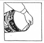
The plastic liner may be carefully peeled out of the inside of the tube.
