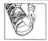
Some tubes are waxed outside. If you plan to paint the outside of the tube, a light sanding will remove some of the wax and make painting easier.
