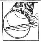
The diameter of the telescope tube should be about 2" larger in diameter than the diameter of the objective mirror.
