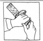
Bevelling the corners so the shingles won't split when the position of the spider is adjusted in the tube.
